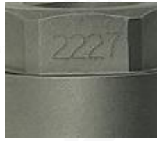
Diesel Pump Overflow Valve Engraving
